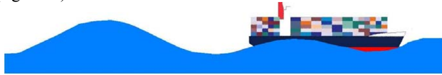
Fig.1.23 Vessel sailing in following waves, large wave approaching from stern
