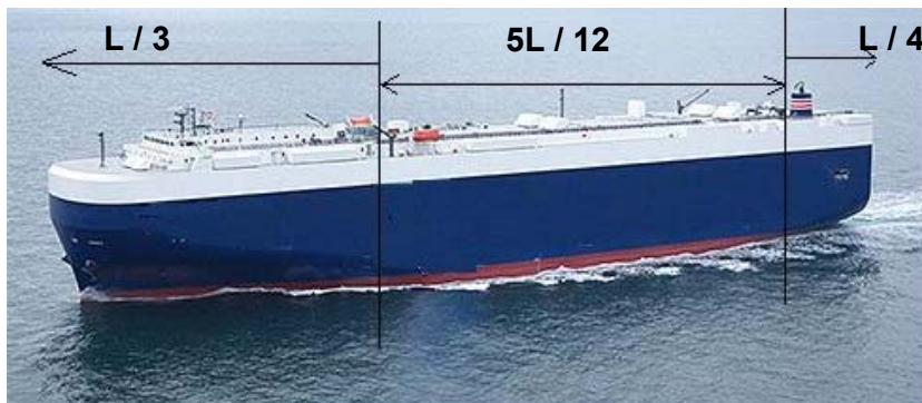
Fig. 2.21 Fractions of the ship's length, car carrier ship
